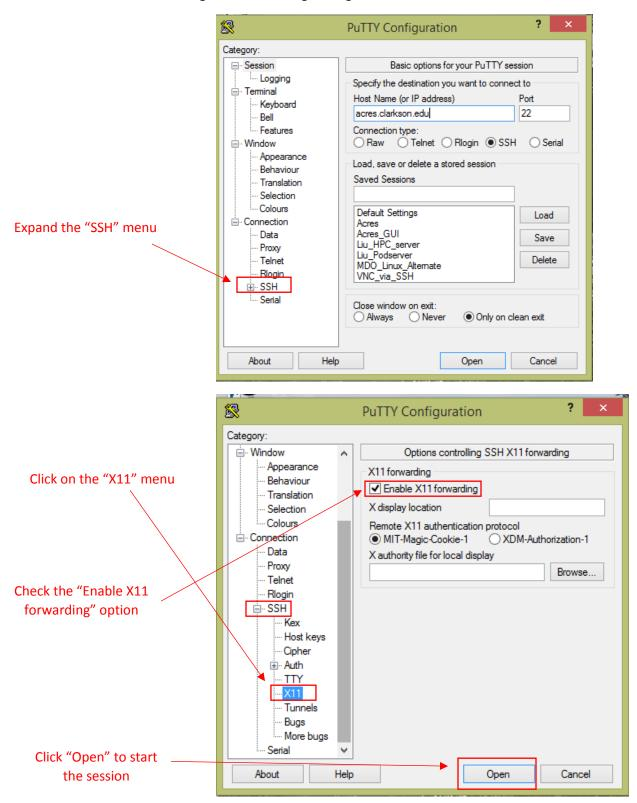
After logging in to ACRES, you can start the GUI application from the command line, and the GUI window should appear on your screen. An example of this is shown below, using MATLAB:
